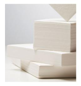
The key characteristics that help us to define the right paper grade are the thickness, the basis weight and the capillary rise (absorption speed). Thicker papers allow separation of higher quantities while lower capillary rise is more suitable for higher resolution.
