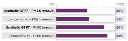
**Synthetic GT F7** is a true F7 / MERV13 filter media reaching >99% removal efficiency of particles with a diameter higher than 5µm.
