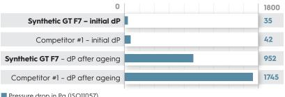
**Synthetic GT F7** reduces energy consumption and can extend the filter lifetime by a factor 2 in pulse jet configuration.
